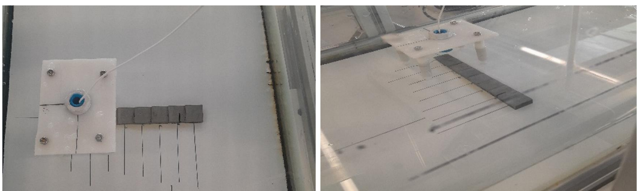
Figure 9 Wedge ultrasonic measurement setup in underwater conditions; Left: Front view, Right: Side View
