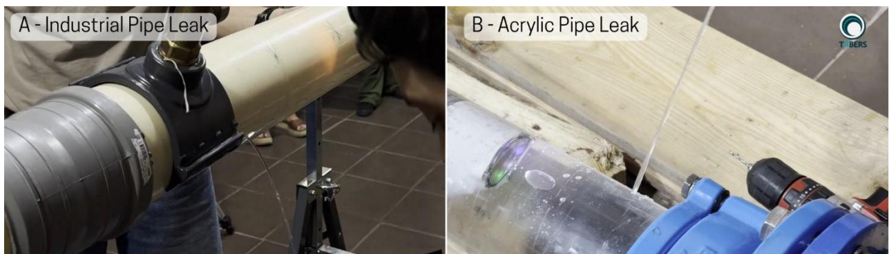
Figure 22: Two defects were demonstrated in the workshop. PE/PVC Pipe (Left) for demonstrating the end-to-end process and Transparent Acrylic Pipe (Right) for demonstration purposes.
