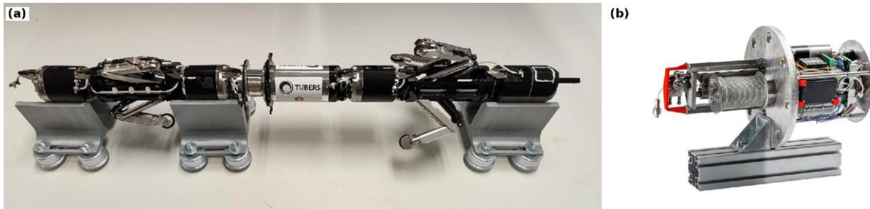
Figure 2: Snake-like robot: (a) UT module integrated into a shortened robot configuration, (b) 20 m tether system with spool and connector
