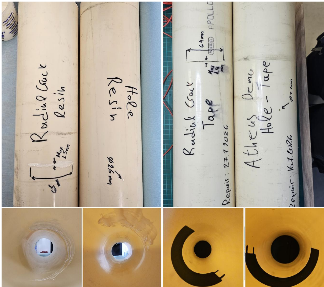
Figure 29: Repaired pipe specimens sent to Brabant Water for Leakage Testing.
