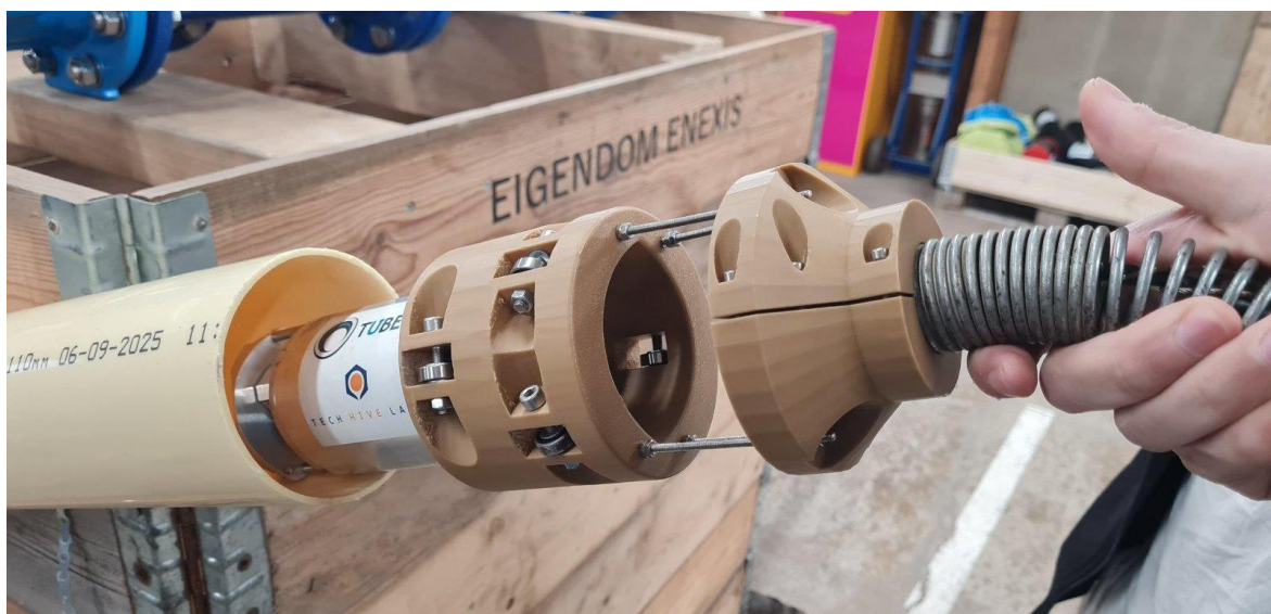
Figure 16: VITENS Preliminary Trials - UT module mounted on the VITENS push-rod system with a custom adapter
